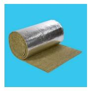
Rosewool Blanket (RKB series) is a good flexible rolled product, mainly made from natural rock such as basalt and dolomite. On request, the rock wool blanket can be water repellent, and also can be faced with aluminum foil, glass tissue or glass cloth on one side or both sides.
